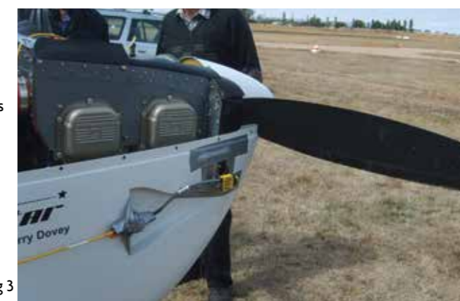
vibration sensor and phototach on an IO-320 engine
